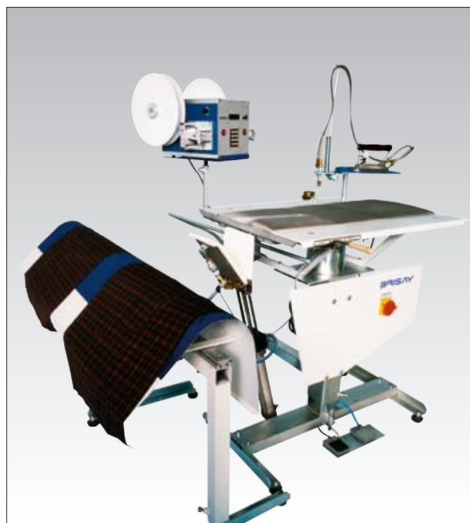
BRI-110 E/101 Ironing table for front part seams (incl. iron BRI-1) • Special ironing surface with slit for chest: prevents a damage of the chest area • Unloading station*: Optional separate stacking of left and right front parts / Increases productivity • Table extension* (additional place of deposit): Improves workstation layout • Programmable tape dispenser BRI-10 for 2 rolls* (automatically cuts fusing tape to preset lengths): Improves work station layout Further advantages 1 2 5 8 9 10 11
