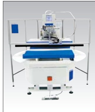
BRI-585C/101 Back centre- and side-seam pressing machine (180 carousel) incl. iron BRI-1
