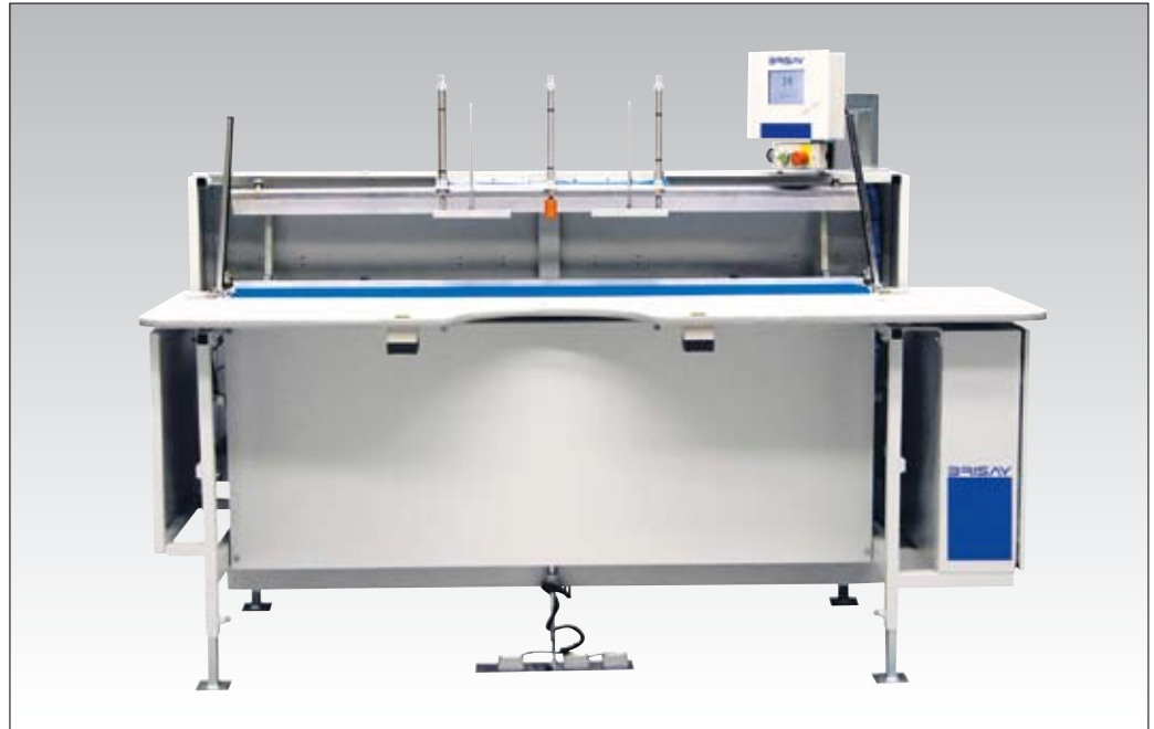
Operation: Folding and pressing of jacket hems
