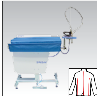
BRI-158/101 Ironing table for back center- and side-seams (incl. iron BRI-1)
