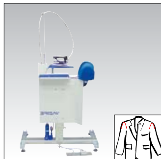
BRI-165/101 Ironing table for sleeve head seams (incl. iron BRI-1)
